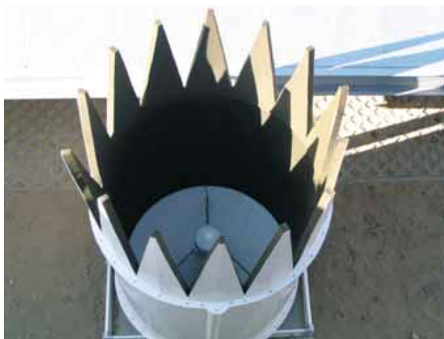
The Radio Acoustic Sounding System (RASS) provides virtual temperature profiles, pictured is one of the four RASS units.
