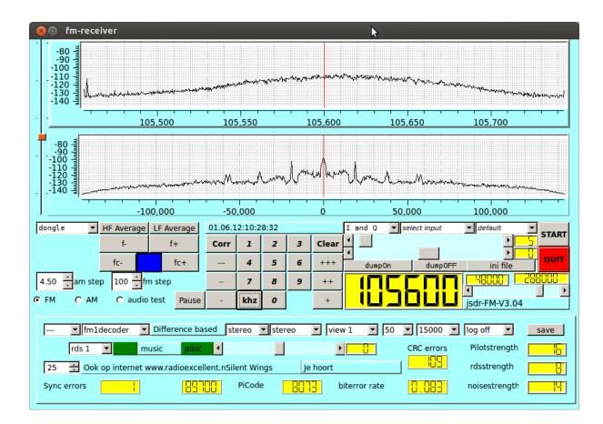
The software, when connected to the pmsdr kit, supports a continuous tuning range from 100K to 165 MHz. The lower frequencies mostly provide AM broadcasts, the FM band obviously provides FM broadcasts. When connected to the DAB stick, a continuous tuning range from app 45 MHz to 1700 Mhz is supported.
