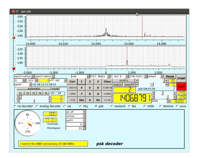
A variety of decoders is available. For each of the decoders a separate subscreen (the bottom part) is shown, with selectors, sliders and buttons specific to the selected decoder. The screen will appear when selecting the decoder.
