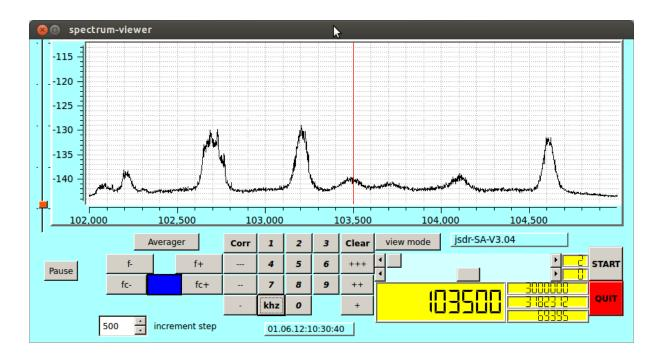
The figure shows a spectrum of a part of the FM broadcast band, with a spectrum width of 3 MHz.
